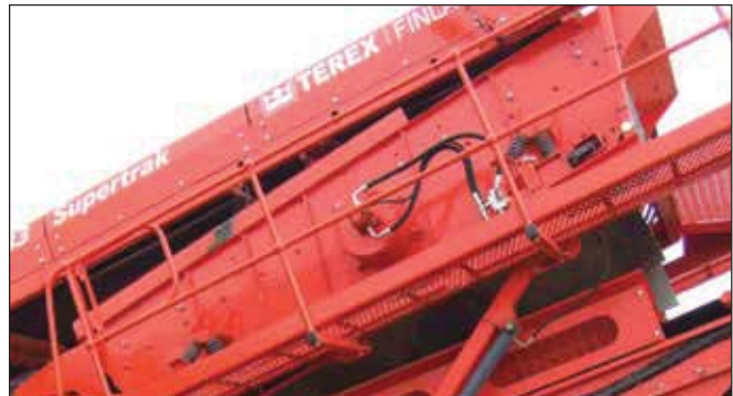
Screenbox with all round catwalks access
